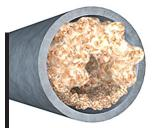
Waste Accumulates in your pipes causing slow, or even clogged, drains. This accumulation, if left unchecked can lead to slow running drains or clogged drains.
